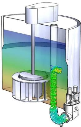
The following symptoms on a flotation plant indicates that a back pressure pipe is required:
