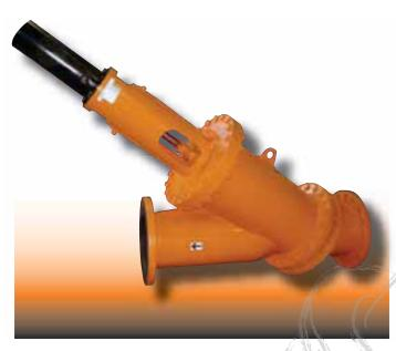
The **DUAL** valve operates on the discharge side of the pump. As the flow through the pipeline starts or stops, the ball automatically rises or falls, opening or closing the valve. The handwheel is there to lock the ball in position. *The handwheel can be used to isolate, but with back pressure.* The Dual valve can work in the horizontal and vertical position.
