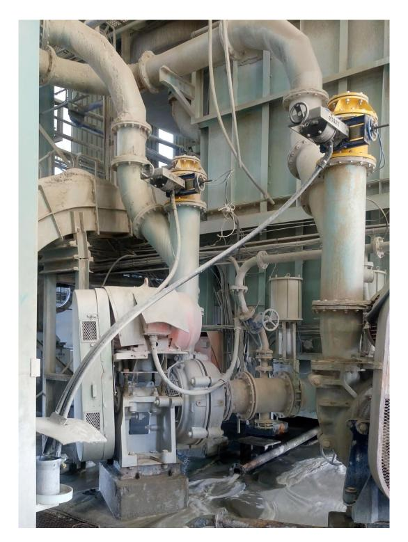
**Offset Pressure Pipe Sampler**
