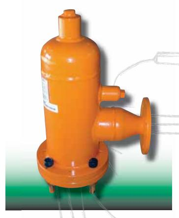
**DUAL**'s Pump Protection Valve has been designed and manufactured to provide protection against excessive fluid temperature rise, within the pump housing. Low flow conditions can cause flashing, cavitation, vibration, bearing failure and damage to mechanical seals and pump housing. The DPPV valve is fitted to the suction side of the pump.
