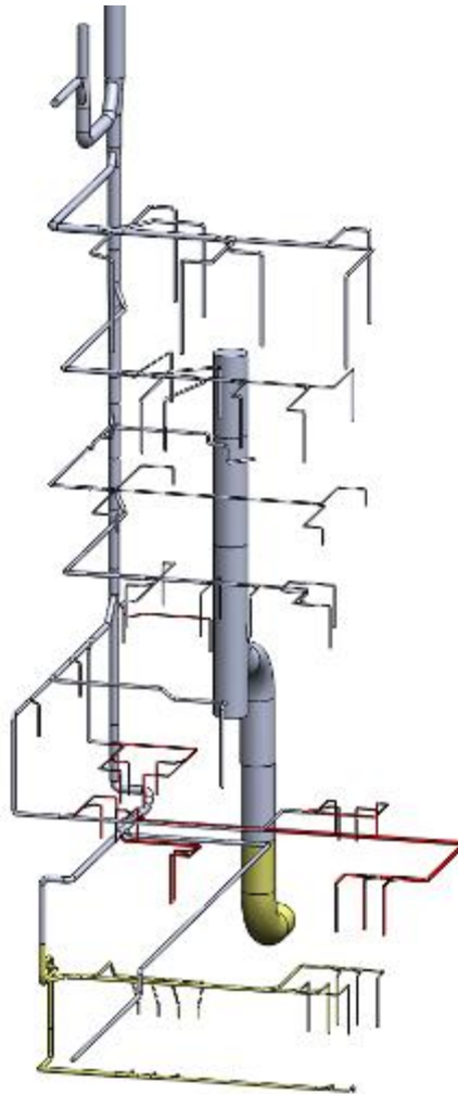
Figure 10: Partial View of Dust Extraction System
